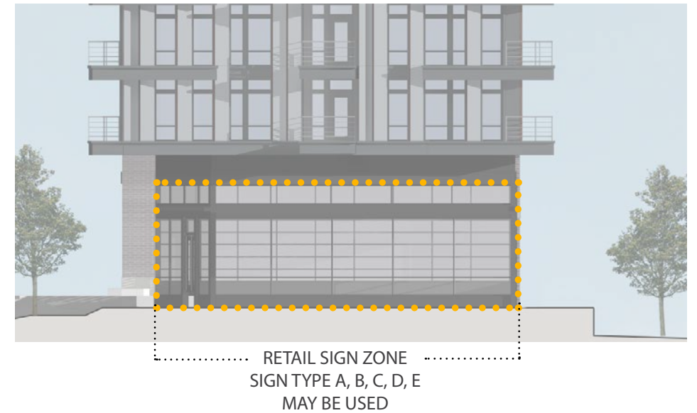
1 - PARTIAL WEST ELEVATION
